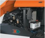
Engine swing out system makes servicing the engine simple by allowing easy access to all sides of the engine.
