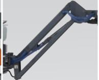
All hosing and lines to the basket and jib are protected by covers and placed out of impact areas to keep downtime to a minimum while allowing easy service access.
