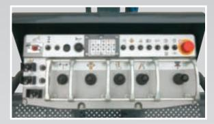
**Ergonomically designed platform controls** are simple to use and well protected. Features rugged hand grips, which also serve as protection to the joystickl controls.
