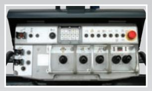
**Dual steering joysticks** allow easy positioning of the unit and zero turning radius. Allockable steel control panel cover is standard on all models to limit damage and unauthorized use of the equipment.
